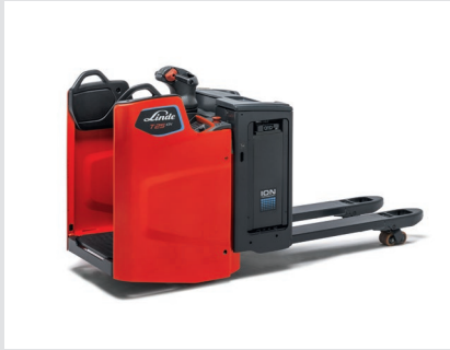
Operator remains safe within the chassis contours
