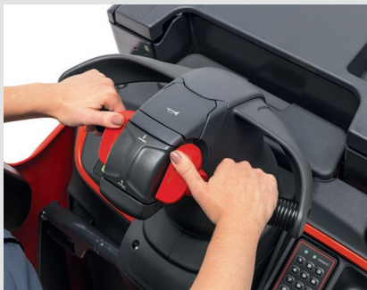
Ergonomic, height adjustable control handle
